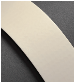
Carlisle's Sure-Weld TPO – 60 Weeks (No Failure)
